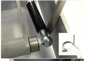
Install front end of new Gas Spring by snapping in place using Flathead Screwdriver, noting orientation as shown and repeat for other Gas Spring if necessary
