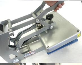
Lower handle to rest heater on lower platen
