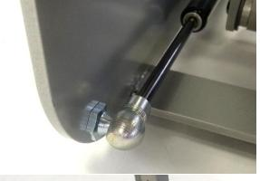
Lift up press and install back end of Gas Spring by snapping in place with fingers as shown
