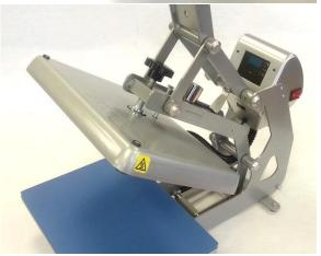
Operate lift handle up and down to verify proper operation of new Gas Springs
