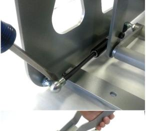
While holding lift handle up, gently pry old Gas Spring rear end off of its ball joint using Flathead Screwdriver as shown and repeat for other Gas Spring if necessary
