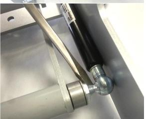
Gently pry old Gas Spring front end off of its ball joint using Flathead Screwdriver as shown and repeat for other Gas Spring if necessary
